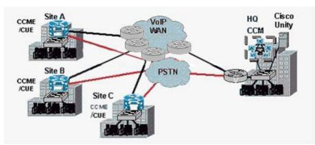
In the network shown in the exhibit, VoIP is used over the intranet WAN to facilicate all voice communications between all sites. Calls out of the intranet are made direct via the PSTN at each site.
