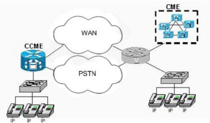
Refer to the VoIP network shown in the exhibit. On which link in the network would the QoS mechanism link fragmentation and interleaving (LFI) most likely be deployed?
