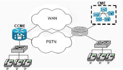
Refer to the VoIP network shown in the exhibit. On which link in the network would the QoS mechanism Compressed Real-Time Transport Protocol (cRTP) most likely be deployed?
